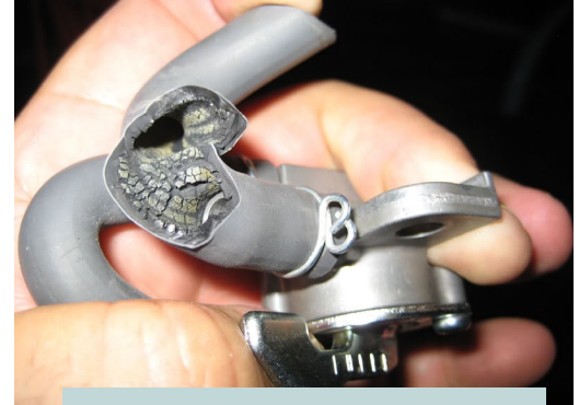
Fuel line damaged by Ethanol
